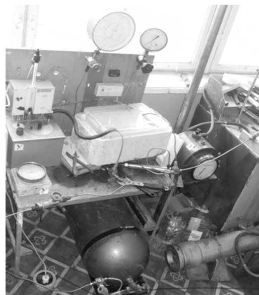
1 – model; 2 – source of gas; 3 – reference cell; 4 – pressure gauges; 5 – manifolds; 6 – input valve; 7 – output valve; 8 – вакуумний насос; 9 – gas meter; 10 – thermo bath; 11 – temperature sensor
