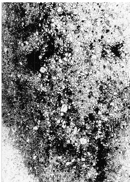
**Figure 1.** Fine-grained sandstone with chlorite-glaucanite clay cement
