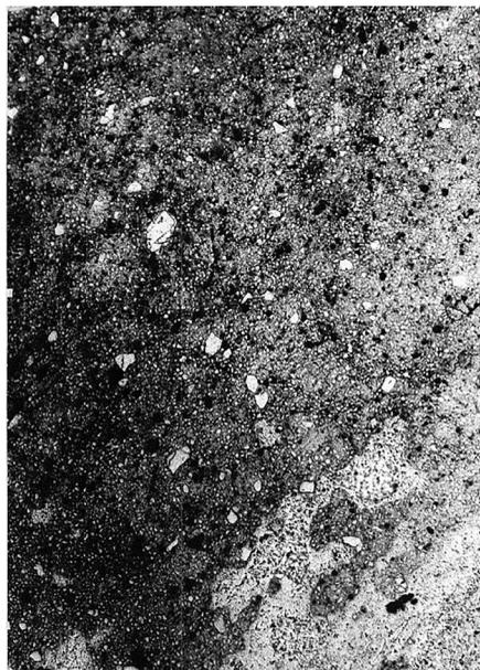
**Figure 3.** Silty sandstone with hydromica clay cement
